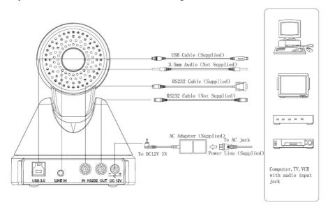
Step2. Power connected to the Camera, the front panel power lamp light.
