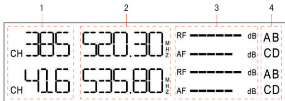
1. Channel number 2. Working frequency 3. Audio and signal level 4. Frequency group
