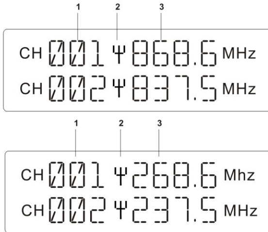
1. Channel display 2. Receive sign display 3. Frequency display
